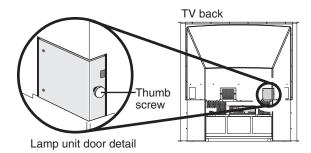
WARNING: The lamp unit door is provided with an interlock to reduce the risk of electric shock and excessive ultraviolet radiation. Never defeat its purpose or attempt to service without removing the lamp unit door completely. Failure to follow this WARNING may result in death or serious injury.
